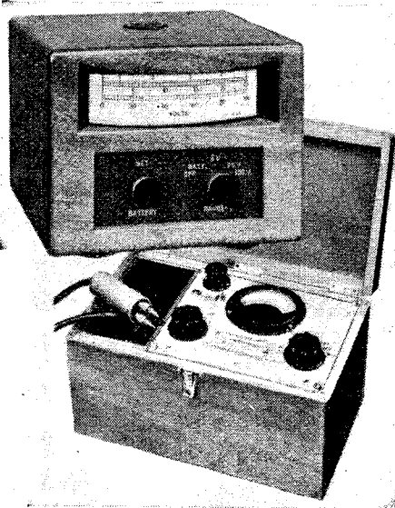
Salford Type BW218 valve voltmeter with vertical scale and (below) peak diode voltmeter Type BW211 for frequencies from 20 c/s to 200 Mc/s.
